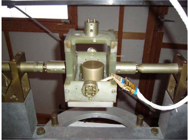
Fig. 7 Sensor in fixture which defines the mechanical reference system with a precision of 10 arcsec
