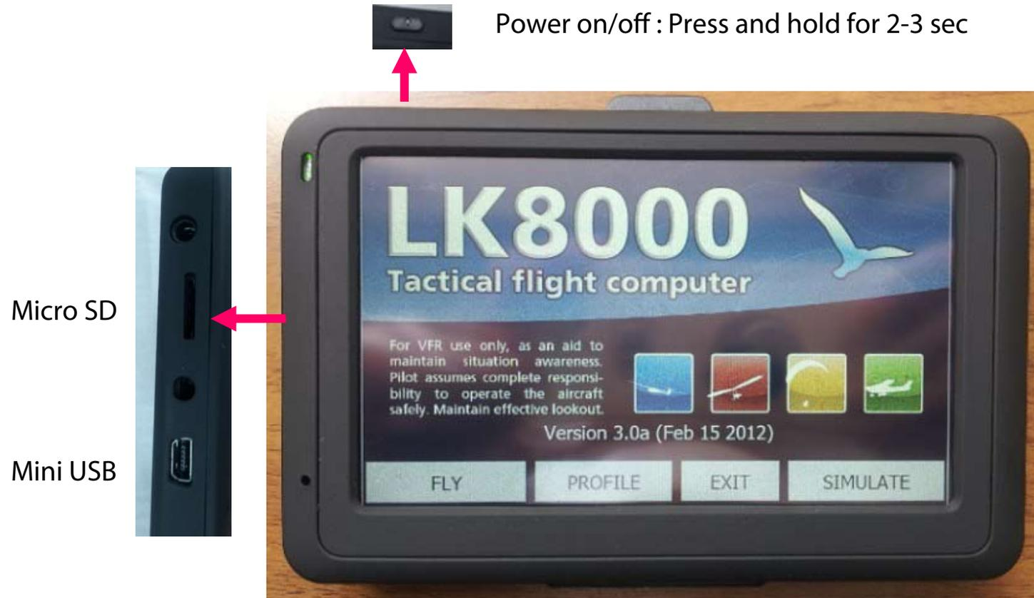
The V2 runs on the operating system Windows Mobile v6.1 which is based on Windows CE 5 kernel.
